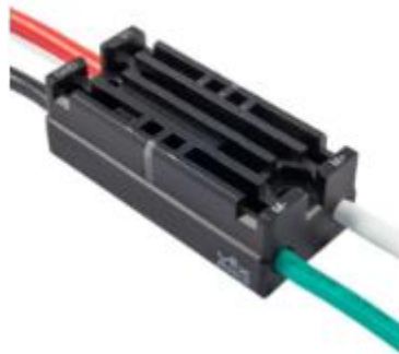
Figure 2.12 A typical Victor SP speed controller.
