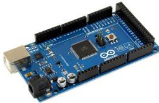
Figure 2.3: A typical Arduino Mega-2560 microcontroller board.
